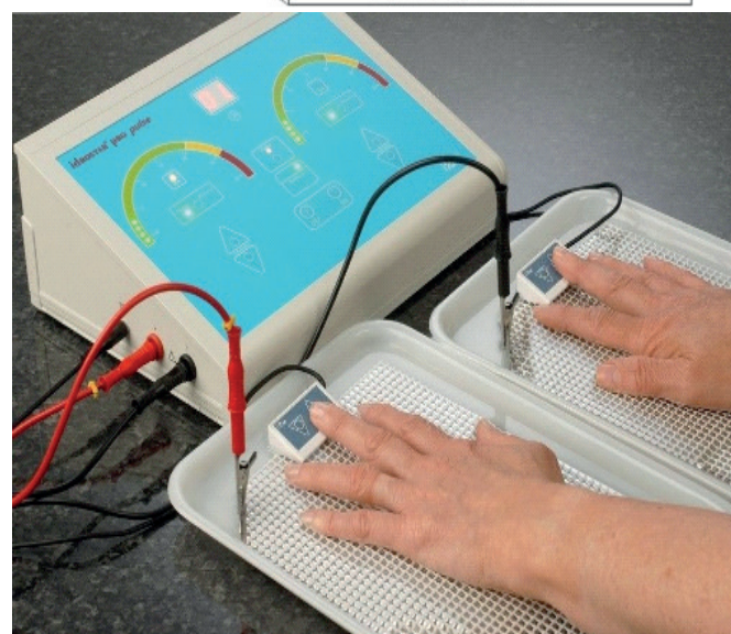
Figure 4. Diagrammatic representation of iontophoresis
