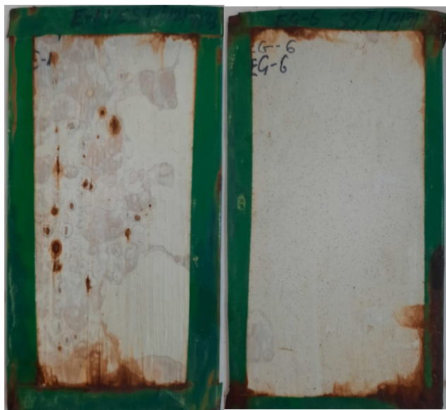
(A) Cardanol epoxy paint sample. (B) 1.0% Graphene-cardanol epoxy paint sample.
