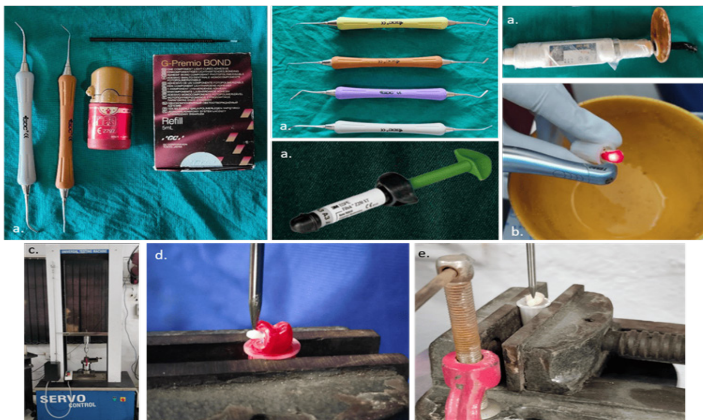
Figure 3 a. Armamentarium;b. application of laser to samples; c. Universal Testing Machine; d. & e. jig with 4x1/8th inch with cross head of 1mm/min
