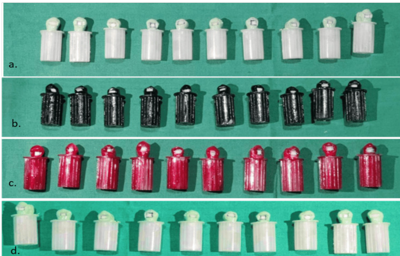
Figure 1 Specimens divided into 4 groups: a.Control; b. Group E (Er: YAG); c. Group N (Nd: YAG); d. Group D (Diode laser)
