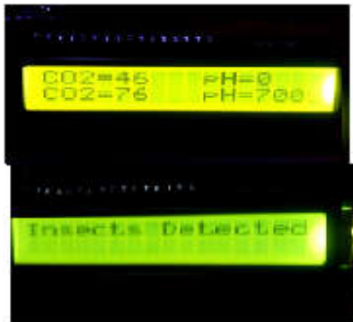
Figure 3.3 Values retrieved by the sensors and Message indication about the detection of White Grub displayed in LCD
