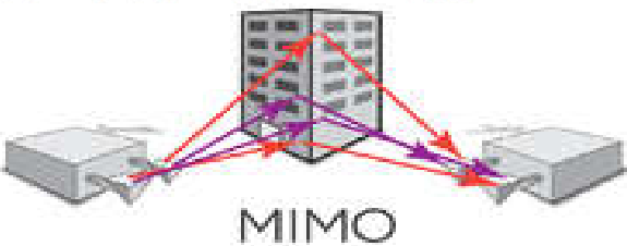
Fig 2 (a) MIMO uses Multipath propagation to exploit link capacity. (b) SM system model.
