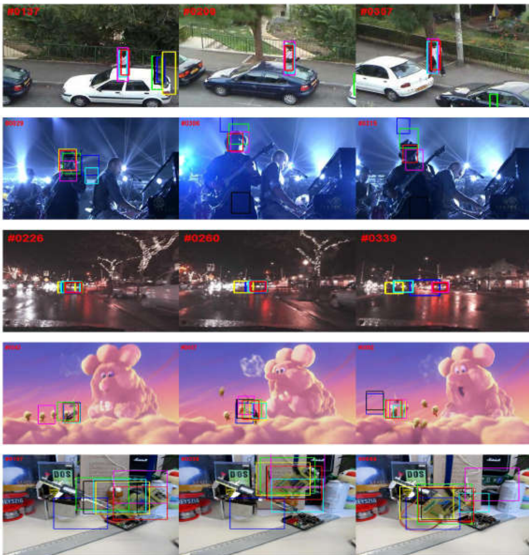
Fig 1 Challenges during tracking in real-world environments, occlusion (woman), abrupt motion (shaking), illumination change (carDark), pose variation(Bird) and complex background (board). We use blue, green, black, yellow, magenta, cyan and red rectangles to indicate the tracking results of the IVT [9], ASLA [10], OSPT [11], CT [12], Struck [13], DLT [14] and the proposed method, respectively.
