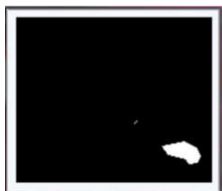
(e) Foreground Mask with shadow removed and morphological operation performed Vehicle Segmentation Process
