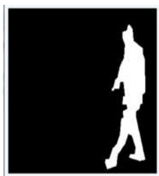
(e) Foreground Mask with shadow removed and morphological operation performed Human Segmentation process
