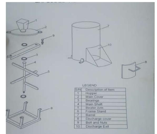
Figure 5 Exploded view of the machine
