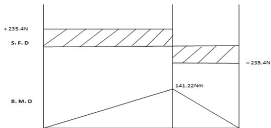
Figure 2. Shear force and bending moment diagram of the drive shaft in static position.
