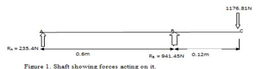
Figure 1. Shaft showing forces acting on it.
