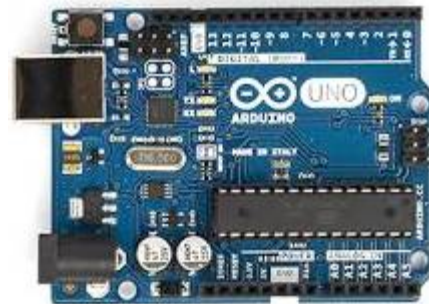
Fig 2 Arduino UNO board can interface to various expansion boards and other circuits.
