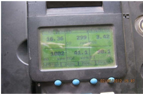
Fig. 3 Flue gas analyser showing NO x emission readings
