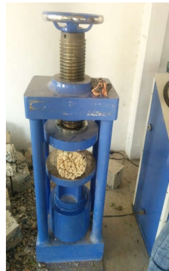
Fig 2 Split Tensile Strength Test
