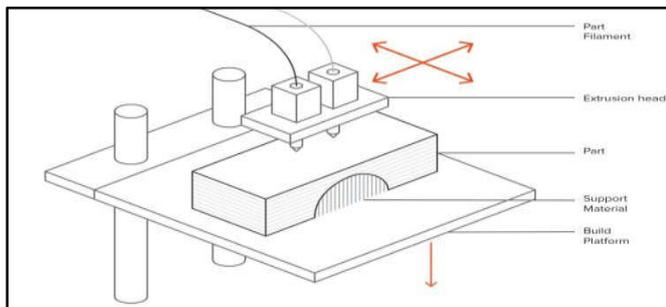
Figure 9 FDM printer setup
