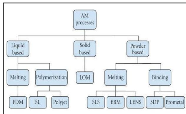
Figure 8 Classification of Additive Manufacturing process
