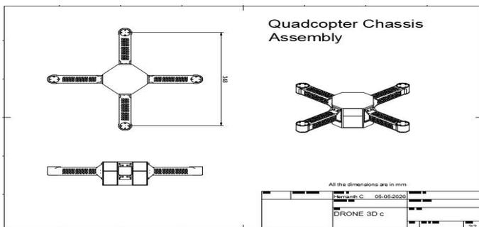
Figure 3 Quadcopter assembly 2D drawings
