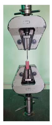
Figure 3 Load applied on the teeth in Universal Testing Machine
