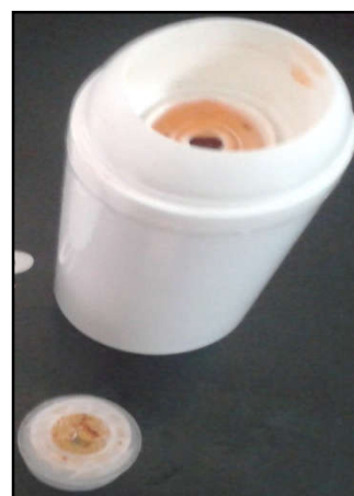
Figure 13 Problems of blockages in metered dose container From table 15 it can be observed due to blockages (figure 13) weight variation per pump/actuation occurred. Therefore, it was decided to fill in sachet which would also ensure accuracy and ease of dispensing, it can be also added on biscuits, yoghurts, breads, etc.
