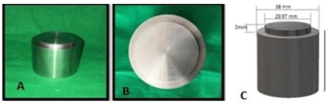
Fig 2 Metal Die- A and B Metal Die; C-Metal Die with Measurement specifications
